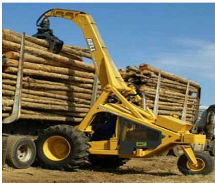
Three-wheel logger required to do loading, sorting and unloading of Sawlogs
